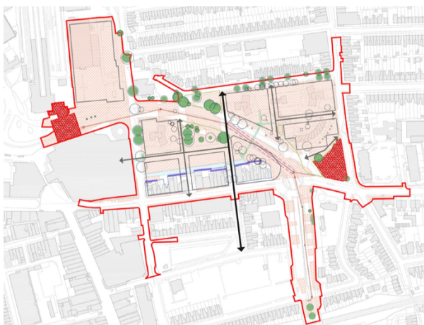
Extract of LDA Constraints Report, which informed the siting and extent of Phase 1A Buildings, particularly utility retention /diversions, highways assets and works, Essex Street access, existing mature tree retention and extensions of existing street network.
